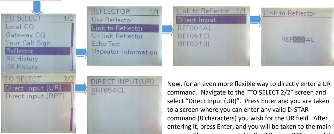
Now, for an even more flexible way to directly enter a UR command. Navigate to the "TO SELECT 2/2" screen and select "Direct Input (UR)". Press Enter and you are taken to a screen where you can enter any valid D-STAR command (8 characters) you wish for the UR field. After entering it, press Enter, and you will be taken to the main screen with your command in the TO area. PTT to send it.
